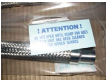
Assembly that has been cleaned and bagged for oxygen service.
