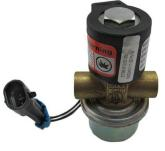
The Model ET98 is an electrically operated safety shutoff valve suitable for high pressure up to 315 PSI for LPG liquid, LPG Vapor or Natural Gas Vapor. It is normally closed Straight-Through Lockoff, opened with 12V DC.
