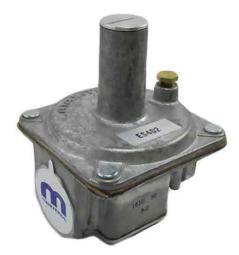
The IMPCO IMP Series of Regulators are low pressure, dry gas regulators intended for use with propane or natural gas. Typical applications include all types of stationary, gas-fired appliances and equipment utilizing a low-pressure gas supply. The IMP Series regulators feature a unique conical valve design, which permits low resistance straight-through flow. This design provides high flow at low pressures and enable the regulator to handle large capacity appliances with limited supply pressure.
