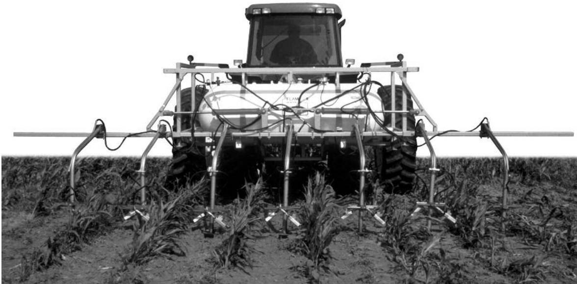
6 RU Shown Here With Optional Hydraulic Tool Bar
