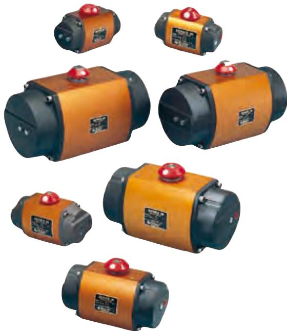
The Series F39 Pneumatic Actuator design is based on the opposed rack-and-pinion principle utilizing piston guide rods to guarantee part alignment. The fully supported guide rods minimize friction and wear between the pistons and the body bore.
