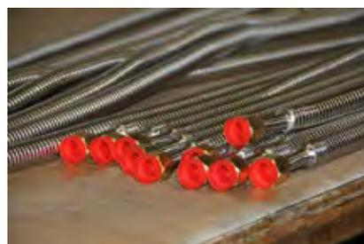
Assembly that has been cleaned and bagged for oxygen service.
