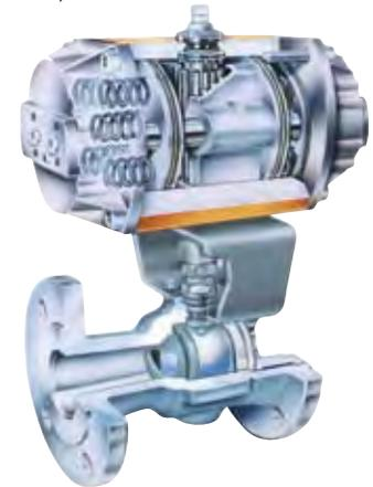
Piston tilting is prevented due to unique guide rods that always keep the pistons parallel with each other and perpendicular to the cylinder. This feature enables the Series 39 actuator to match the performance of diaphragm actuators in terms of high resolution. Internal friction is reduced with a nickel acetate-coated cylinder, low coefficient-of-friction acetal resin bearings and a special permanent lubricant with corrosion inhibitors.
