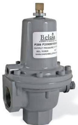
The Type P289 Back Pressure Regulator functions as a high flow relief valve with an adjustable set point. The P289 can be used in place of a standard relief valve to provide protection against over pressurization in the downstream system. The design of a large diaphragm area and a pitot tube booster allow the valve to respond quickly and relieve the excessive pressure smoothly, especially in low-pressure settings.
