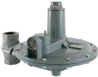
The Type P143 pressure regulator is ideal for propane. Uses include commercial, residential and light industrial for burners and unit heaters. The P143 has an internal relief device and is available in the low pressure cut off (LPCO) version.
