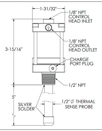
ALL LTAP PROBES ARE SUPPLIED WITH SINTERED BREATHER INSTALLED IN THE CONTROL HEAD **OUTLET PORT AND A 1/4"** TUBE BY 1/8" NPT BI-Lok **DUAL FERRULE FITTING** FOR THE CONTROL HEAD INLET. THIS FITTING IS SUPPLIED LOOSE.
