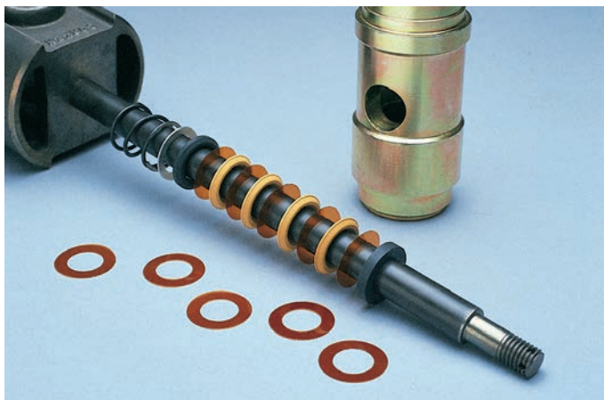
Crosshead guide, piston rod, packing barrel, K-ring spacers and packing set.
