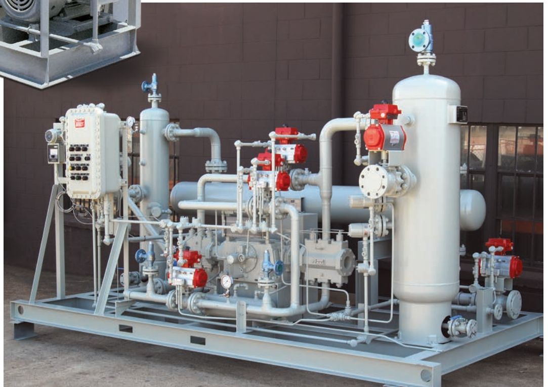
Right: HG602CE-109C two-stage compressor package designed for LPG sphere evacuation. This package can operate in single-stage and two-stage mode for deep evacuation. This package can also be used for propylene and other products.
